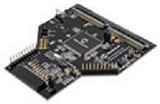
This PCB (ATMXT1189TDAT-I2C-PCB) is for the evaluation and development of Microchip maXTouch applications using the ATMXT1189TDAT Touchscreen Sensor IC.
